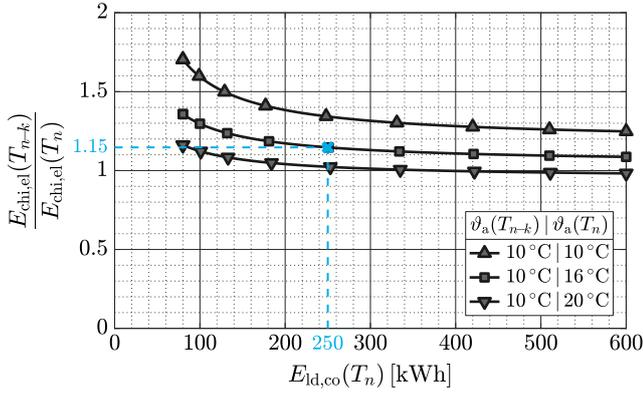
Fig. 4. Ratio of electrical energy consumption versus  $E_{ld,co}(T_n)$  for different ambient temperatures.
