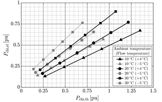
Fig. 3. Linearized load profiles of a compression chiller.
