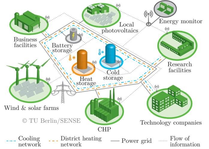
Fig. 1. Scheme of a multi-energy microgrid.
