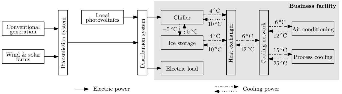
Fig. 2. Block diagram of multi-energy system with cooling supply system.
