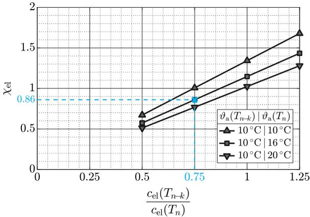
Fig. 6. Cost ratio versus electricity price ratio for different ambient temperatures, a cooling demand of 250kWh and parameters from Table I.
